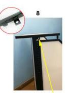
Place counter on top of bar & situate holes evenly. Tab should face guest NOT bartender. Insert bolts in holes & tighten.
